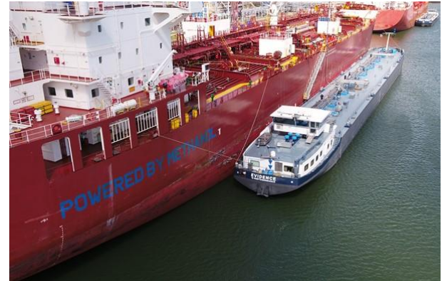
World's first barge-to- ship methanol bunkering operation In partnership with the Port of Rotterdam, Vopak, TankMatch and NYK Shipping
