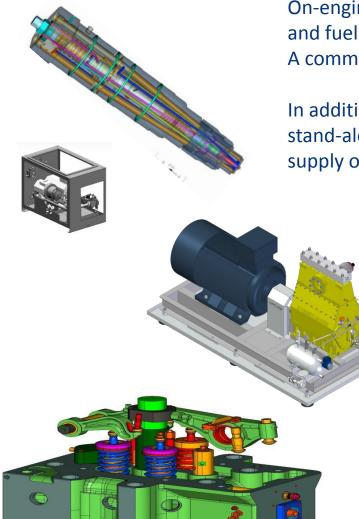
On-engine scope is limited to exchange of cylinder heads, fuel injectors and fuel plungers in existing fuel pumps. A common rail system for methanol injection will be added on the engine.
